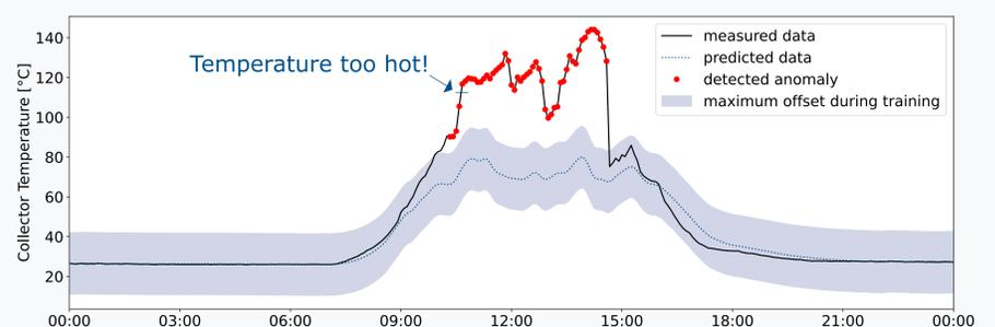
The figure displays measurement data showing the temperature of a collector (black line) and predictions provided by our algorithm (blue line showing predictions and blue area encoding the maximum offset observed during training). Half an hour before a stagnation occurs at approximately 10:30 o'clock, our algorithm already detects anomalous behaviour (red dots). This would have been enough time to react to the anomaly and prevent the stagnation.
